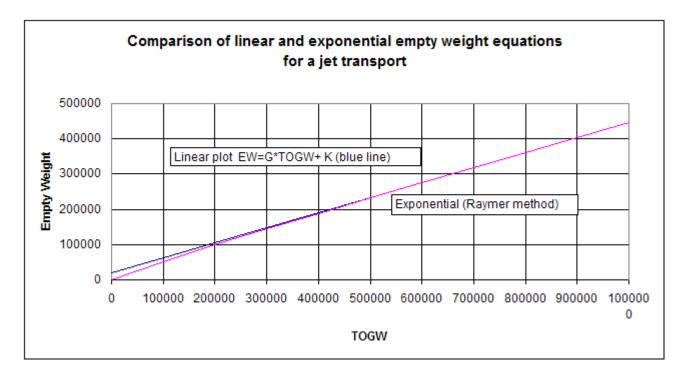
Fig 3.3.1 Comparison of Linear and Exponential Empty Weight Equations
