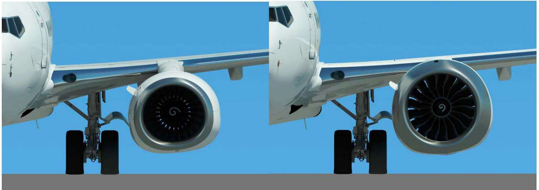
Figure 1. Boeing 737NG (left) and MAX (right) nacelles compared. Source: Boeing 737 MAX brochure.
