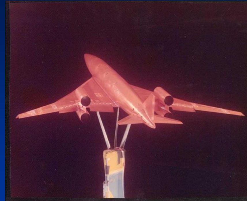
Over/Under Engine Concept in Low Speed Wind Tunnel
