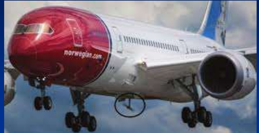
Deployed RAT on 787
