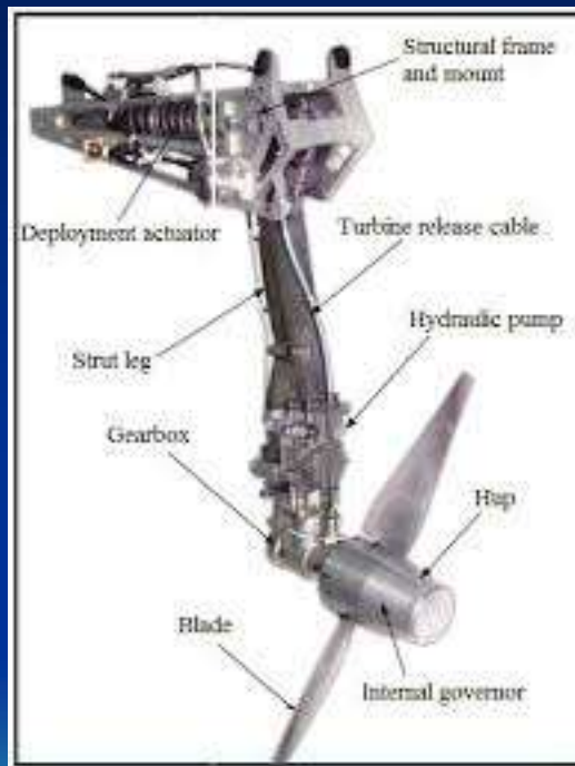
A-380 RAT (1.63 m dia. propeller)
